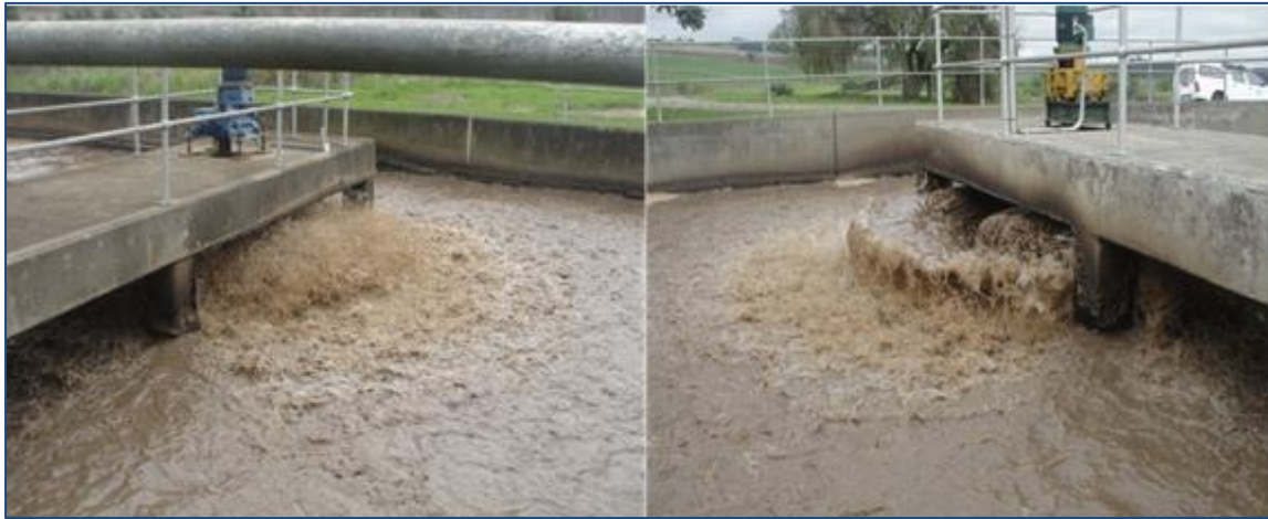
Figure 19.56 Different Mechanical Surface Aerators in Cool Air Reactor 1 and 2.
