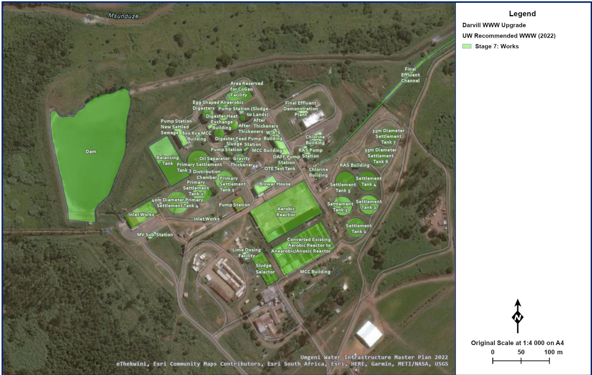
Figure 19.41 Upgrade of Darvill WWWW.
